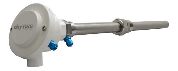
The ST carbon probe incorporates a SIRO<sub>2</sub> all ceramic oxygen sensor. The probe comes with a 25mm Inconel sheath for extended life and additional protection. It is used for measurement and control of oxygen sensitive environments at high temperatures. The sensor operates in situ, and measures oxygen concentration in real time, without the need for expensive gas sampling, or gas extraction equipment.
