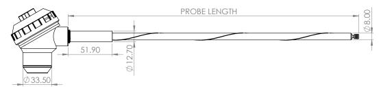
**FLS** – Comes with a full-length ceramic sheath running the entire length of the probe. The ceramic sheath provides a measure of protection to the sensor tip from direct exposure to corrosive and high velocity gases, reducing overall wear. A 1" BSPT or NPT compression fitting is available for this sheath option.
